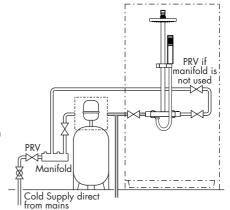
It is recommended that the cold supply be taken from one of the outlets of the manifold directly to the shower as an independent supply.
