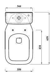
**Special notes**Pan fixes to floor using side fixing bracket supplied with pan.
