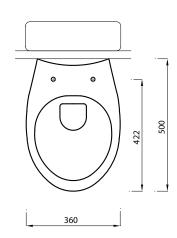
**Special notes**Pan fixes to floor using side fixing bracket supplied with pan.
