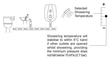
Water inlet pressure fluctuations due to other draw offs (e.g. flushing toilet) will cause the showering temperature to increase.
