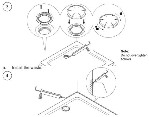
a. Apply silicone sealant in accordance with the manufacturer's instructions to seal the shower tray to the wall.
