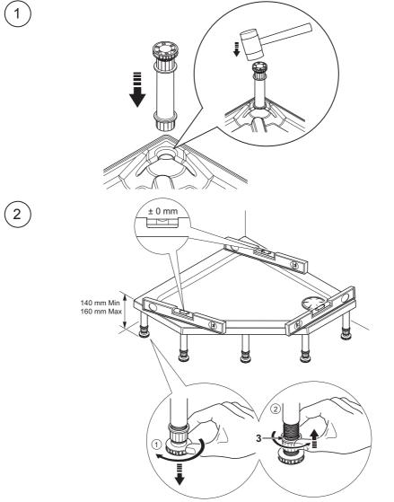
a. Make sure that the shower tray is level, adjust the legs as necessary.
