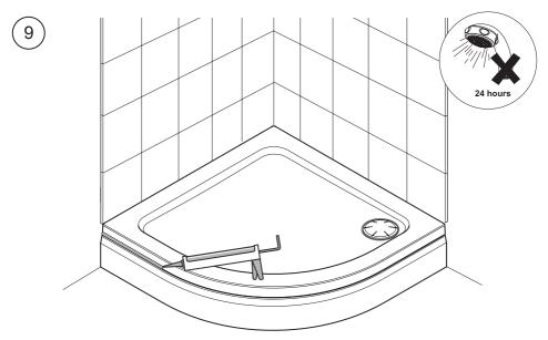
a. Apply silicone sealant in accordance with the manufacturer's instructions to seal the edge of the panel to the shower tray.
