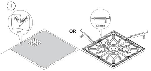
a. Install the shower tray on a bed of sand and cement or silicone sealant.
