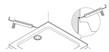
a. Apply silicone sealant in accordance with the manufacturer's instructions to seal the shower tray to the wall.
