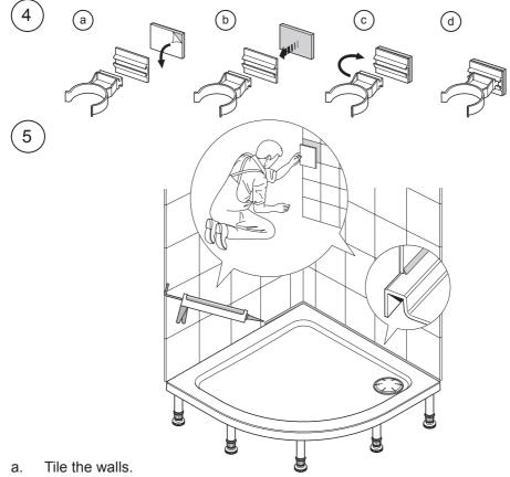
b. Apply silicone sealant in accordance with the manufacturer's instructions to seal the shower tray to the tiled wall surface.
