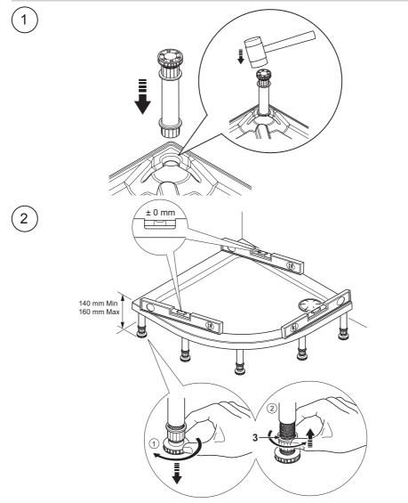
a. Make sure that the shower tray is level, adjust the legs as necessary.
