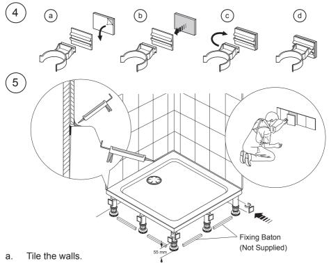
b. Apply silicone sealant in accordance with the manufacturer's instructions to seal the shower tray to the tiled wall surface.
