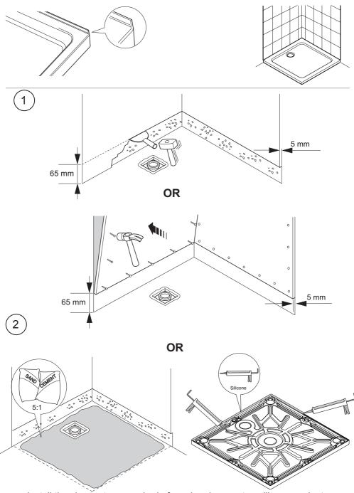
a. Install the shower tray on a bed of sand and cement or silicone sealant.
