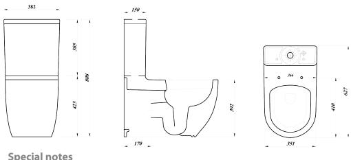
**Special notes** Pan fixes to floor using side fixing bracket supplied with pan
