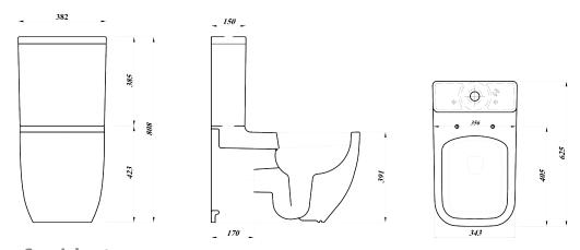
**Special notes**Pan fixes to floor using side fixing bracket supplied with pan.
