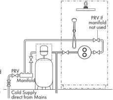
Flow regulators are required for installations where a PRV is not fitted to ensure simultaneous demand is accounted for.
