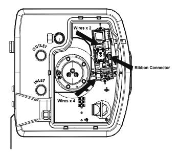
Figure 13: iBD Wiring removal
