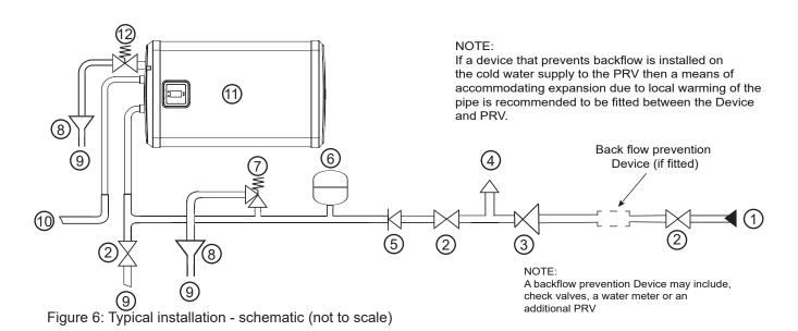
Item Description 1 Cold Water Mains in 2 Service Valve (not supplied) 3 Pressure Reducing Valve 4 Balanced Cold Water Draw Off 5 Check Valve 6 **Expansion Vessel** 7 Expansion (Pressure) Relief Valve 8 Tundish 9 To Drain (Waste) 10 Hot out Water heater 11 12 Temperature and Pressure Relief Valve
